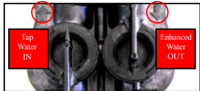
Inlet and Outlet Bypass Valves Open
